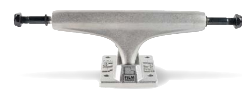
INVERTED KINGPIN INVERTED KINGPIN ALLEN SYSTEM SILVER POLISHED HANGER & BASEPLATE BLACK MEDIUM BUSHINGS 5.25, 5.5 & 6" 135, 145 & 165 MM
